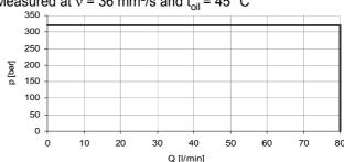
The operating limits were determined using coils at operating temperature and 10% under voltage. The operating limits given are for applications with two flow directions. For flow in only one direction, the operating limits can be lower.
