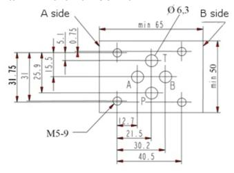
Mounting screws: M5 x 30 DIN 912-10.9
